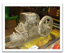
Yep, that's about an inch or so of dried bird poop encrusting this engine. Some of our engines were found in similar conditions, though not as extreme as this example. Surprisingly, the babbitt bearings, valves and rings looked brand new, the valve faces and seats having a mirror-like finish! Very strange for an engine in this condition, but the restorer found clues as to what happened. (That won't be discussed in this article.)
